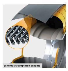
Twisted Steel Belt High stiffness of tire in lateral direction
