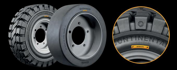
Every vehicle charges electrically while driving, as conventional tires are practically not conductive. This is normally not a problem, yet in some sensitive application areas, uncontrolled electric discharges may cause sparks. That is why we have developed especially conductive versions of our Super Elastic Tires SC20 and MH20, which prevent static charging.
