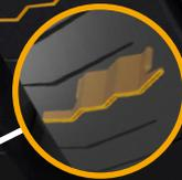
Full-depth pocket sipes at 50% of rib width minimize uneven wear and enhance water displacement for improved performance on wet roads
