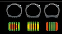
Example: Even pressure distribution at recommended tire pressure of 8.5 bar
