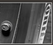
ContiPressureCheck uses a sensor inside the tire to continuously monitor the air pressure and tire temperature.
