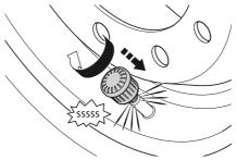
Turn the Valve Cap Sensor an additional quater to half turn to seal the valve steam correctly.
