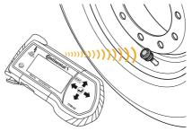
Switch from the user setting "← TIRE SENSOR →" using the left or right arrow key to "← VALVE SENSOR →". Proceed with this selection for each tire based on sensor type.
