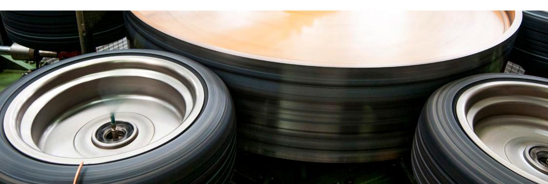
Endurance testing doesn't look at how a tyre wears but what it can actually withstand: When and why does it reach the limit of its structural endurance? In addition to high-speed testing, there are also burst, bead unseating and plunger tests, which are carried out to ensure and document compliance with all regulatory requirements.
