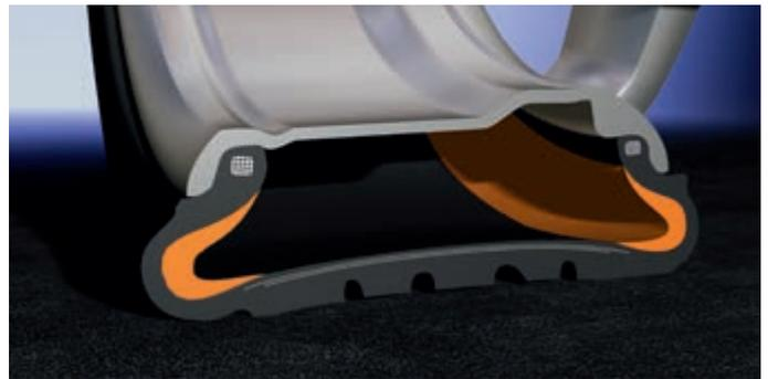
When a puncture occurs with a standard tire, the sidewall can become crushed between the rim and the road causing a potentially dangerous situation. The reinforced sidewall in the self supporting runflat tire prevents this from happening.
