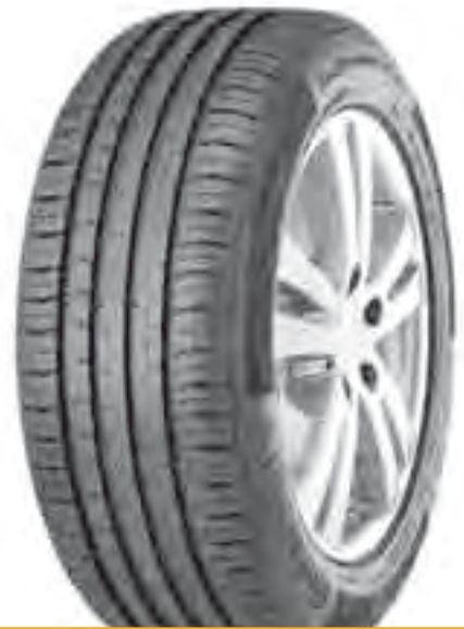
Tyre example: ContiPremiumContact 5, 205/55 R 16 91V.
