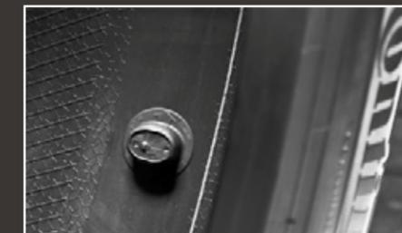
ContiPressureCheck uses a sensor inside the tire to continuously monitor the air pressure and tire temperature.
