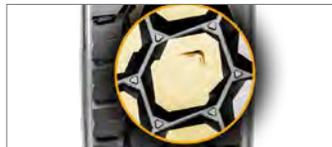
**Diamond shaped lugs** and optimal void volume for excellent traction.
