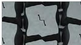
**Patented innovative groove technology** leads to minimal stone retention, extending casing life.
