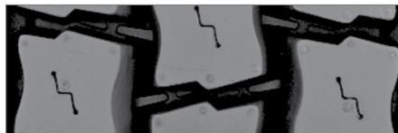
Innovative groove geometry minimizes stone retention.
