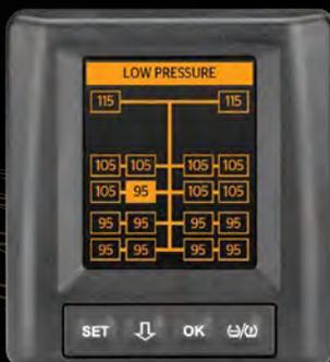
**ContiPressureCheck®** monitors a single vehicle in real-time, alerting the driver to tire pressure and temperature issues via an in-cab display. It is ideal for fleets whose trucks or buses are away from the terminal for long periods of time, and for owner-operators. Fleets benefit from extended tire and casing life, as well as increasing fuel economy and improving safety over the road.
