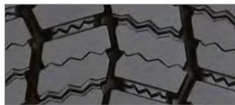
**Directional tread design** with more than 1000 sipes provides excellent traction and lateral stability.
