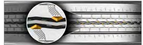
**Pyramidal stone ejection** system integrated into the center groove for added casing protection.
