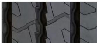
**Zigzag center groove geometry** increases the number of biting edges for increased traction.
