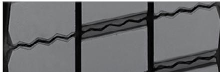
**Narrowed groove widths** result in increased pattern volume which improves wear resistance to guarantee high mileage performance.
