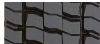
**Chamfered tread block geometry** to withstand higher drive axle torque with reduced drive tire wear conditions such as tearing and cracking.
