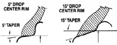
The following diagram shows how beads of a 16" tire will not seat on a 16.5" rim. The beads cannot be forced out against the rim flanges by using more air pressure because this will break the beads and the tire will explode with force sufficient to cause serious injury or death.
