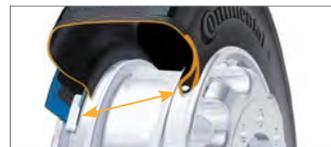
**Improved bead design** for increased durability and resistance to brake heat.
