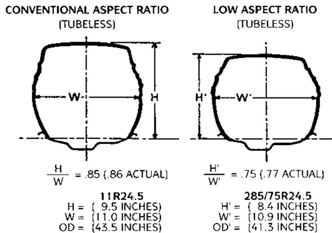
In a tire selection process, it is mandatory that consideration be given to selecting a tire size and load range which at least equals the maximum load requirements by axle position (steer, drive or trail). All highway truck tires have load limits established for tires used in normal highway service. Therefore, when selecting a tire for service, both the carrying capacity and speed implications must be considered.
