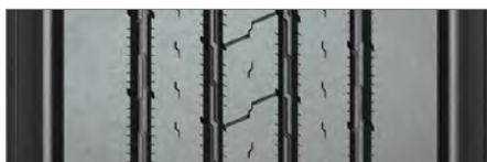
**Improved footprint shape** delivers significant wear improvements for increased removal miles.
