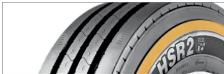
**Sidewall with curb rib** reduces damage from curbing, cuts and abrasions.
