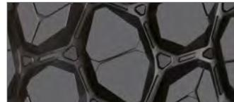
**Alternating groove geometry** and stone bumper system for maximum stone ejection.
