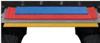
**Rigid belt package** with full width top belt and extra sidewall protection for increased durability.
