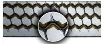
**Self-cleaning tread design and groove geometry** reduces stone retention for enhanced retreadability.
