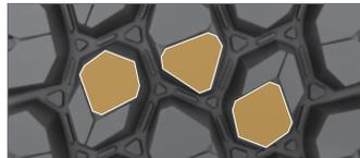
**Diamond shaped tread lug design** and shoulder notches are optimal for chaining.
