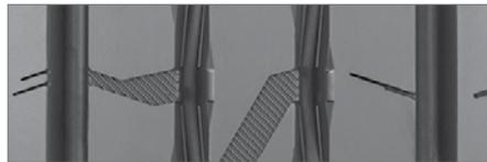
**Narrowed groove widths** result in increased pattern volume which improves wear resistance to provide high mileage performance.
