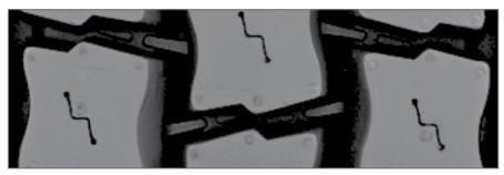
**innovative groove geometry** minimizes stone retention.
