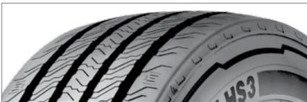
**Two-layer tread construction** combines high mileage performance in the cap compound with significant rolling resistance improvements in the base compound.
