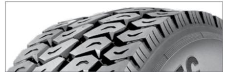
**Thick undertread** resists casing penetration and damage for multiple retreads.
