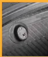
Equipped with TPMS Sensor for accurate, real-time tire pressure and temperature readings • Sensor warranted for 5 Years to minimize disruptions. • Sensor provides true casing temperature allowing preventive actions that make your tire last longer • Avoids valve damage and air leaks by mounting on the inner liner.
