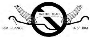
Never assemble a tire and rim unless you have positively identified and correctly matched the parts.
