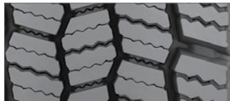
Heavy siping provides **numerous gripping edges** for excellent traction on wet roads.
