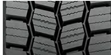
**Directional M + S tread pattern** delivers even wear and traction in both snow or mud.
