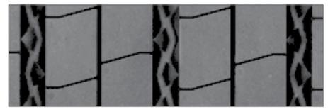
**Patented innovative groove technology** leads to minimum stone retention, extending casing life.
