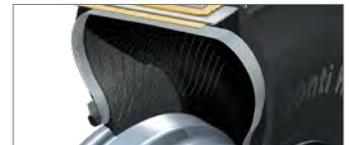
**Maximum sidewall protection** for improved resistance against curbing, cuts and abrasions.
