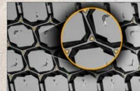
**Self-cleaning tread design** and **miniature stone bumpers** reduce stone retention for enhanced retreadability.
